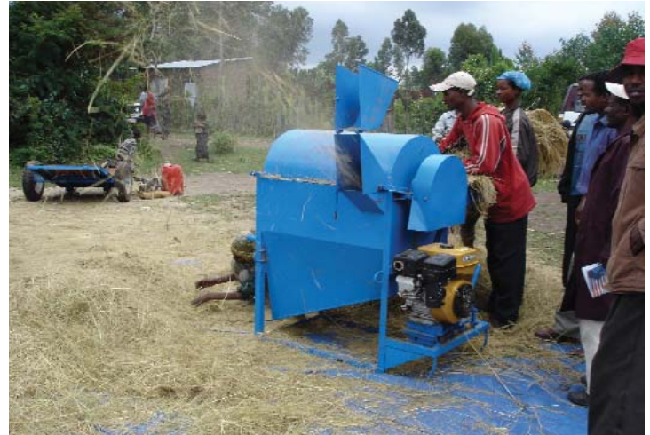
Private tef threshing service provider: this multi-crop thresher was made by a local manufacturer
