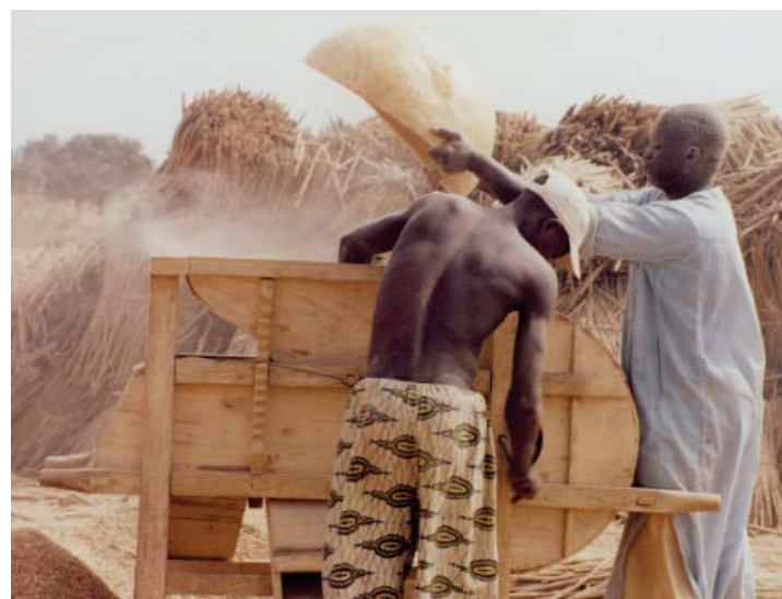
A wooden winnower developed through KNARDA/South-South co-operation is being disseminated to farmers by SG 2000 to curtail the drudgery involved in winnowing of grains
