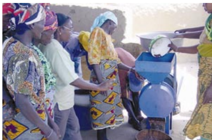
In Northern Ghana, women farmers are using wet-type grinders to process shea-nut butter.
