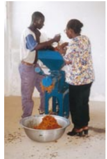
Palm digester in the Technology Village at the University of Cape Coast, Ghana—with Dorothy Ankrah, SAA’s head of agroprocessing in Ghana.
