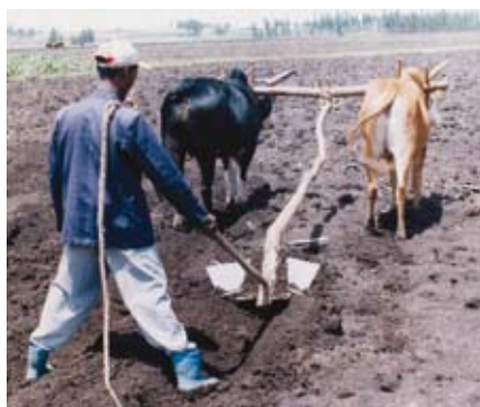
The improved broad-bed maker in operation on heavy vertisol soils.
