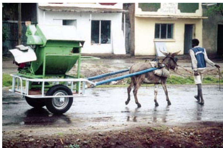
The improved donkey cart is used to transport the IITA-designed multicrop thresher to farmers in Ethiopia.
