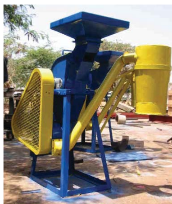
An Alpine grinding mill – one of the new pieces of equipment tested by MSI
