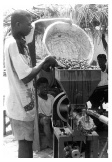
An agroprocessing palm oil digester machine in Ghana.
