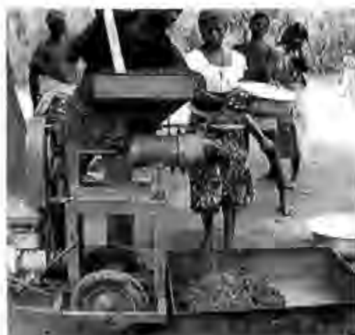
Fig. 4. Left, the grain polisher turned palm oil digester/kernel cracker. Top, augers for grain polishing and kernel cracking (at left) and for palm oil digesting.
