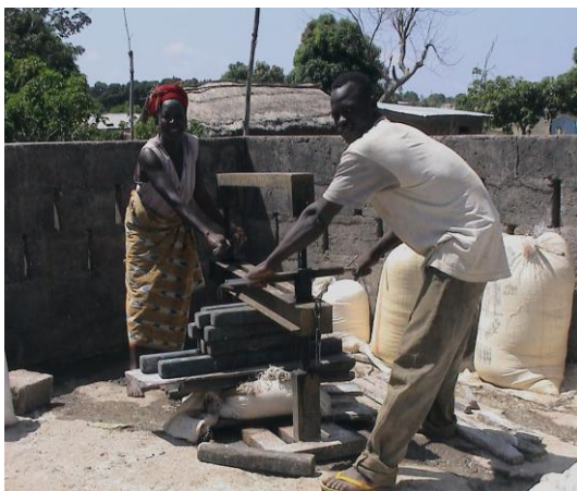
9- The double screw press in Eni eliminated the use of stone piles to dewater grated cassava
