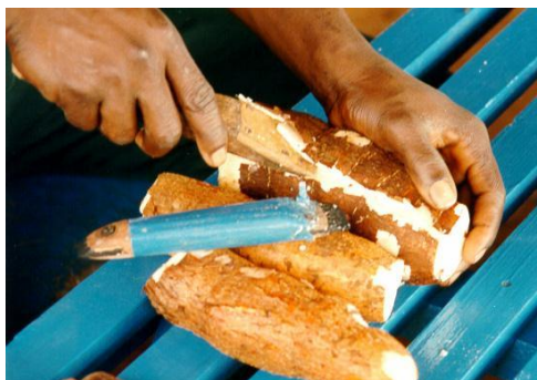
Fig. 7 – Cassava peeling tool to reduce accidents and wastages
