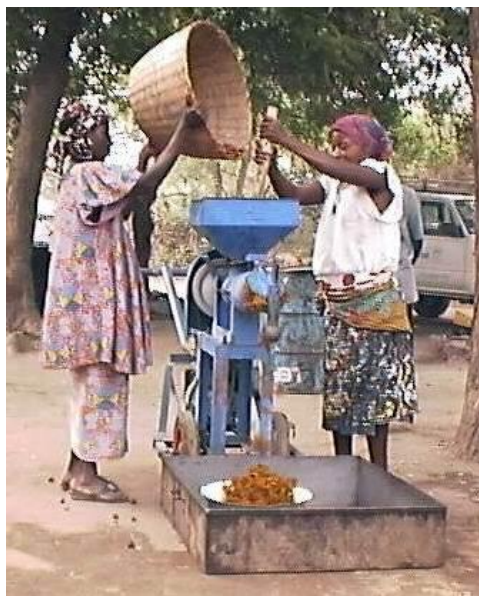
Fig. 30 – Palm oil digester was tested in Atok Village, South of Benin. The difficulty in feeding was due to the height of the machine and inadequate training of operator
