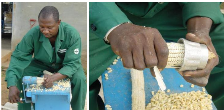
Fig. 14 – Manually-operated maize shellers introduced by the SAA-AP project are simple, low-cost, reduces drudgery and saves time
