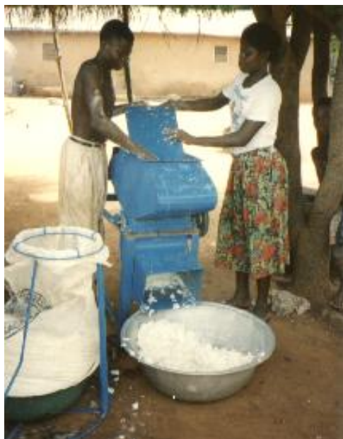
Fig. 8– The portable cassava grater with bagging stand for improve efficiency and reliability
