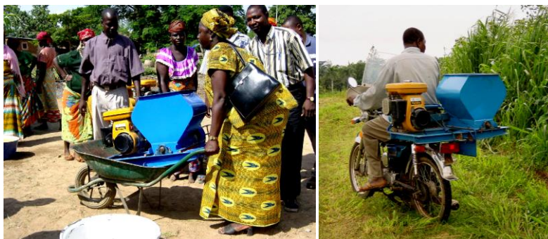
Fig. 20 – The portable grater is giving good income to service providers who now can reach processors in remote villages
