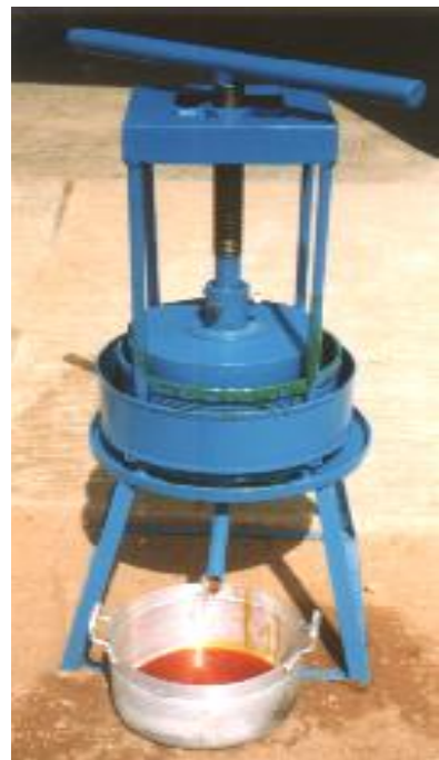
Fig. 19 – The single screw press is easy to operate and maintain. Application: extraction of palm oil, groundnut oil, soymilk, others at the household level
