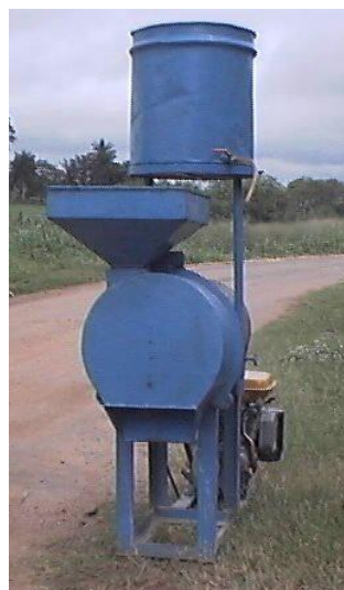
Fig. 17 – The wet type grinder produces fine paste for more efficient extraction of oil or soymilk
