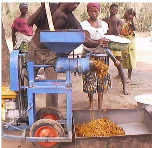
Fig. 26- The grain polisher found its way to palm oil processing yards in Ghana and Benin being used extensively as digester
