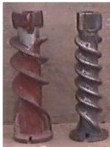
Fig. 27 –Augers developed for cracking palm kernel (L) and for digesting palm oil (R)
