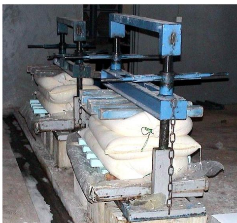
Fig. 11 – The double screw press facilitates dewatering, simple to operate requiring minimum repair and maintenance
