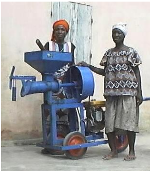
Fig. 18 – The palm oil digester adapted from a grain polisher has transformed backyard palm oil processing into a profitable cottage industry in Ghana
