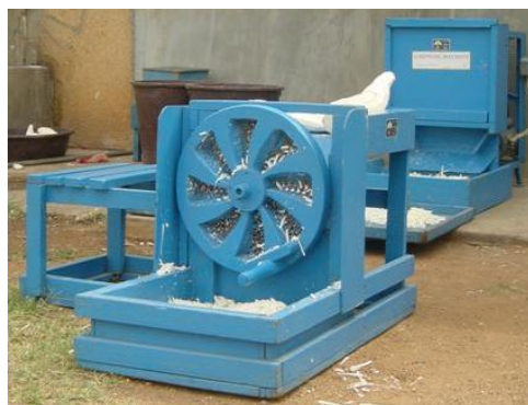
Fig. 13 - The chipper cuts root and tuber crops into thin strips for faster drying
