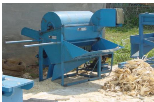
Fig. 22 –The multi-crop thresher with cleaner eliminatethe need for a separate cleaner,is compact and movable
