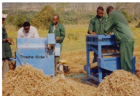
Fig. 16 – The multi-crop thresher and cleaner/ sorter allows quick field handling of crops for subsequent processing
