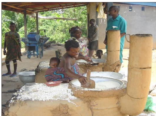
Fig. 12 –Improved IITA gari frying stove (left) and one of the modified local stove (right) eliminate smoke, save fuel-wood and provide comfort to operators
