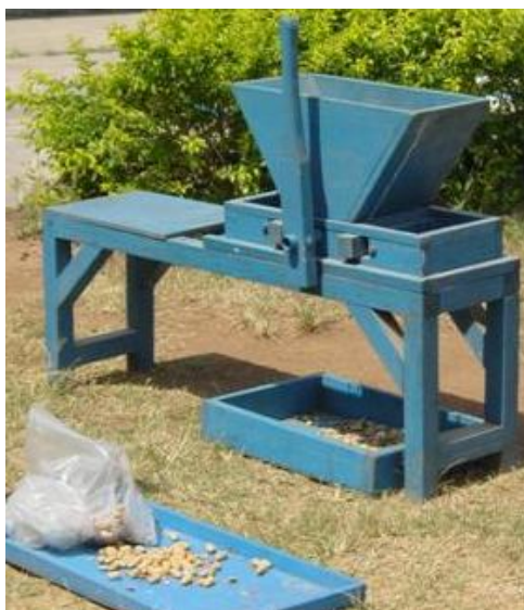
Fig. 15 – The manually-operated groundnut sheller increases shelling rate by almost 90%
