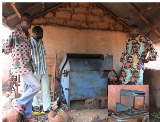
23-The thresher in Atomey is being utilized at full capacity by more than 300 maize farmers. The spring actuated grain cleaner/ sorter (forefront) lasted only for two seasons
