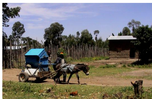
Fig. 23 – The donkey cart developed at STVC is helping to move the thresher to the farmers in their own farms
