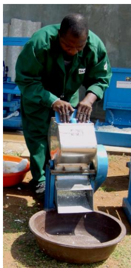
Fig. 21 – The mini-grater opens options to process cassava and other crops
