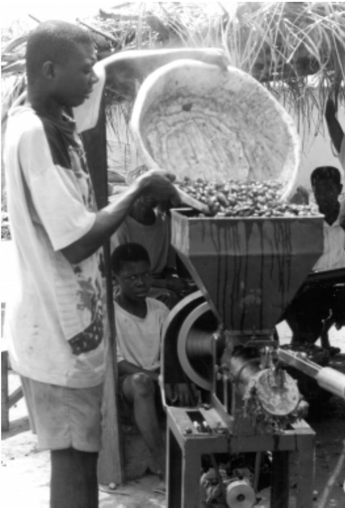
An agroprocessing palm oil digester machine in Ghana.
