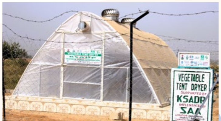
Parabolic solar dryer installed in Dan Dabino market, Bagwai LGA Kano State
